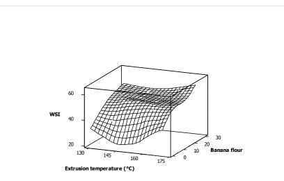
Fig.5. Effect of extrusion temperature and banana flour on WSI of extrudates
