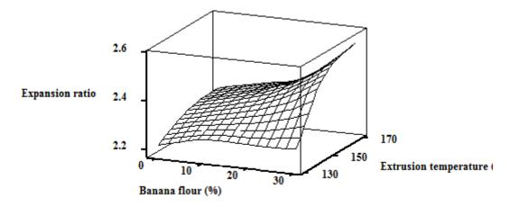
Fig. 8 Effect of Banana flour and Extrusion temperature on Expansion Ratio
