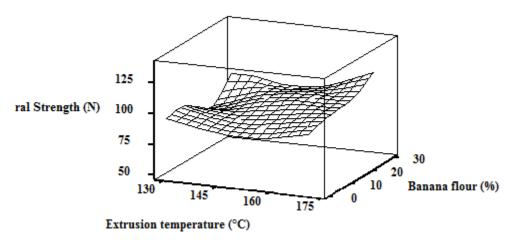
Fig. 11(b) Effect of Extrusion temperature and Banana flour on Flexural strength
