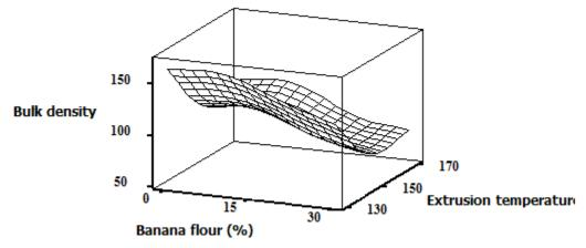
Fig. 9 Effect of Banana flour and Extrusion temperature on Bulk density
