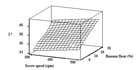
Fig 2. Effect on Banana flour and Screw speed on L\* value of raw extrudates.
