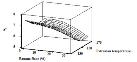
Fig. 5 Effect of Banana flour and Extrusion temperature on a\* value of fried extrudates.
