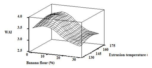
Fig. 6 Effect of Banana flour and Extrusion temperature on WAI
