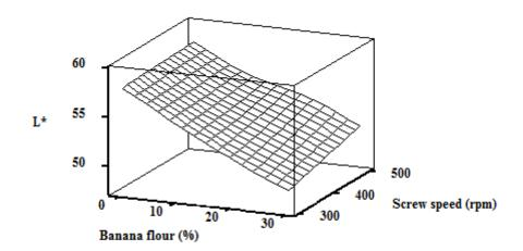
Fig. 4 Effect of Screw speed and Banana flour on L\* value of fried extrudates.
