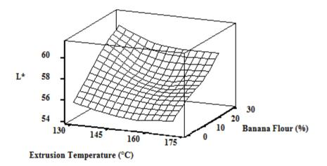
Fig. 1 Effect of Banana flour and Extrusion temperature on L\* values of raw extrudates
