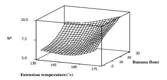
$\it 3ig.2$  Effect on banana flour and extrusion temperature on b\* values of raw extrudates.
