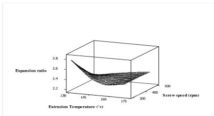
Fig.6. Effect of extrusion temperature and screw speed on expansion ratio of extrudates
